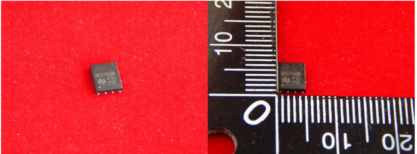
M3056M, N каналный MOSFET (BVDSS - 30V; RDS(on) - 4.2 mΩ; ID - 103A)
