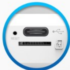
SD CARD SLOT & USB-C POWER (OPTIONAL)
