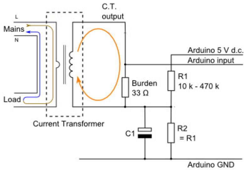
Current Transformer Output: 50 mA rms
