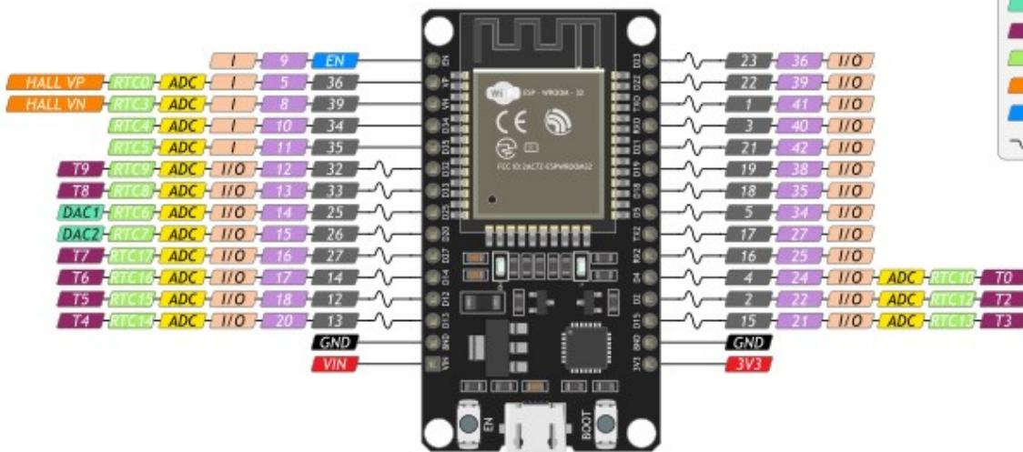
Interface on all GPIO pins: 3×SPI, 3×UART, 2×I<sup>2</sup>C and 2×I<sup>2</sup>S
