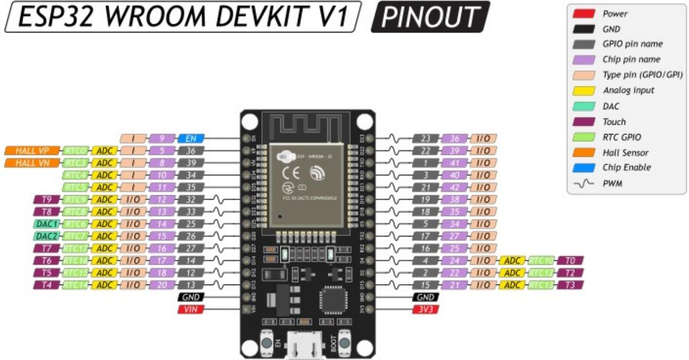
👁 Interface on all GPIO pins: 3×SPI, 3×UART, 2×I<sup>2</sup>C and 2×I<sup>2</sup>S
